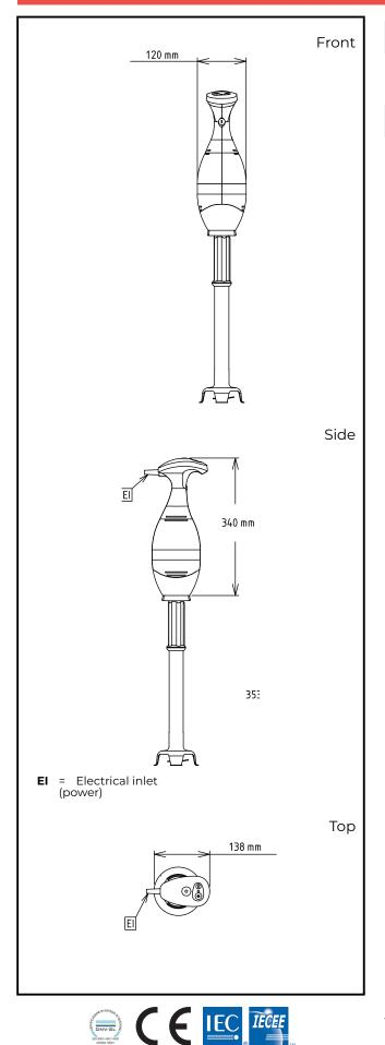
Electric Supply voltage: 220-240 V/1 ph/50/60 Hz **Electrical power max.:** 0.75 kW **Total Watts:** 0.75 kW Key Information: External dimensions, Width: 138 mm External dimensions, 120 mm Depth:
